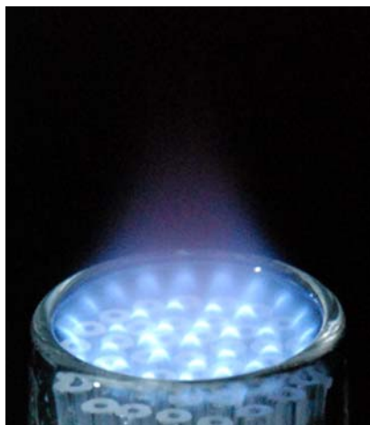
Figure 2. Photo of a stoichiometric methane/air laminar flame stabilized on the multi-jet quartz burner.
