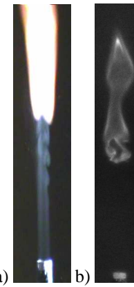
Figure 8: Flow visualizations before the flame (a) and the front flame (b) without the magnetic field for the regime III.
